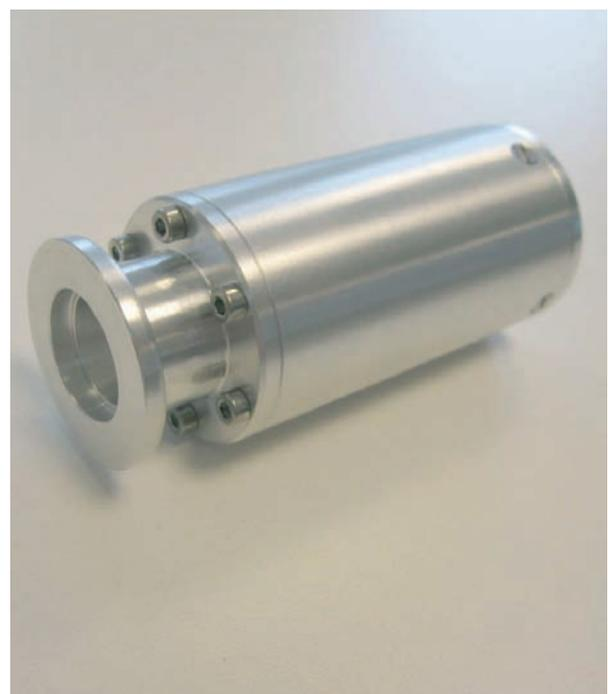
Figure 6: The vacuum-flange-mounted APD detector.
