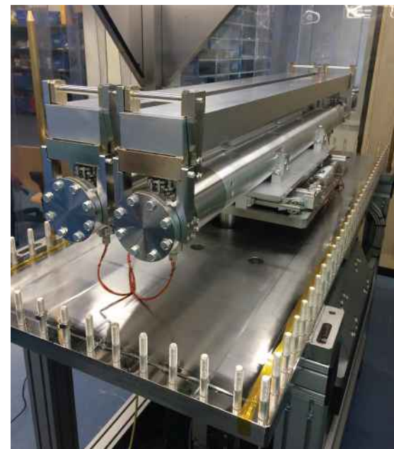
Fig. 2: The new toroidal mirrors system during the factory acceptance tests at IRELEC [2] in January 2020.
