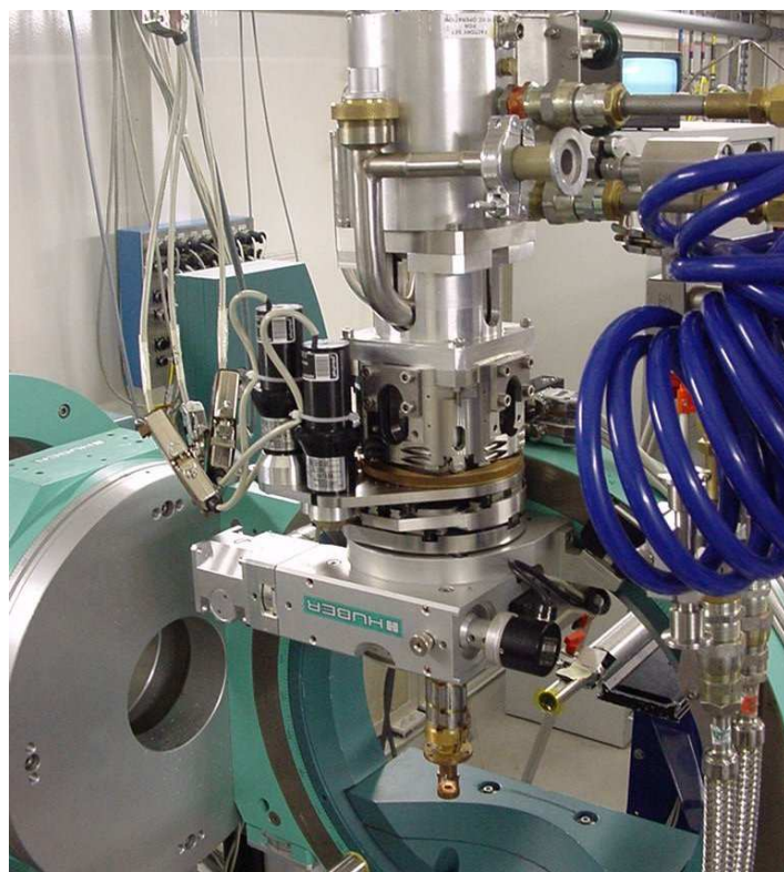
The new xyz cryostat mount, in routine use since March
